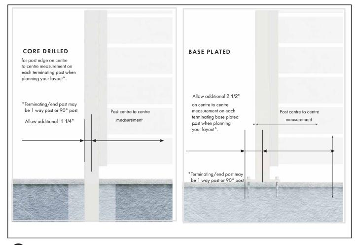
Determine post positions. For simplicity, calculate post positions from centre of post to centre of post. Recommended that post centres do not exceed, in areas of high wind, consider restricted span widths.
