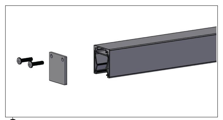
8 Each side frame comes with top and bottom end plate attached. Remove top plate before proceeding to step3.
