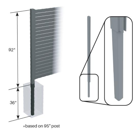
For use when posts need to go into ground more than 24" or fence higher than 6' (will also require side frame). Screw-fix post extender to bottom of post.
