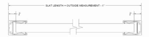
TO DETERMINE SLAT LENGTH, DEDUCT 1"FROM THE OVERALL WIDTH OF THE PANEL, AS SHOWN IN THE ADJACENT DIAGRAM.
