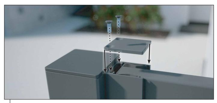
Above final slat, install top plate onto side frames to complete screen.
