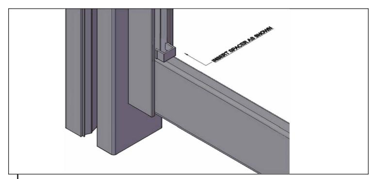
In Snap in spacers above slats on both sides. Add in new slats. Repeat until screen is complete. If no gap is required, stack slats on top of each other without spacers.
