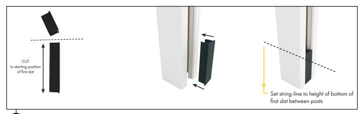
NOTE: For base plate mounted posts on uneven ground/deck, cut one setting block only and place at the highest point of the finished floor line .Then, run a level string line to determine heights of remaining setting blocks before cutting to size.
