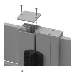
If using 1 or 2 way posts, orient top cap with 2 holes over the slats and screw off top cap into slats.
