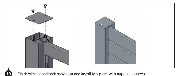
Finish with spacer block above slat and install top plate with supplied screws.
