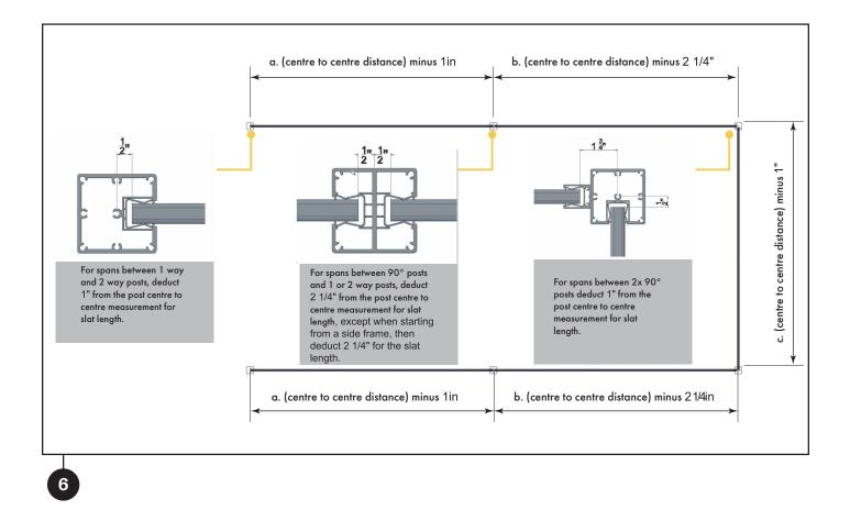
**a.** For spans between any 1 way post and 2 way post combination, slats are cut **1" less** than the centre to centre of posts.
