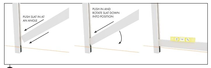
Install first slat in each span. Using spirit level, ensure slats are level.
