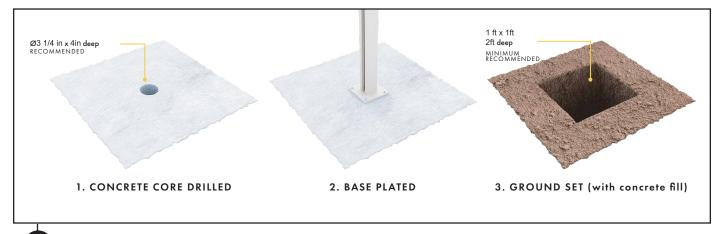
Determine how posts are to be installed:
