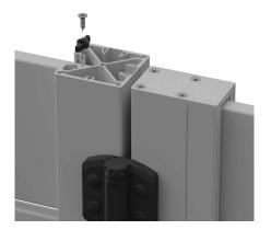
If using 3 way post, ensure there is sufficient space at top of post. Prior to attaching top cap, attach a slat clip to top of top slat.
