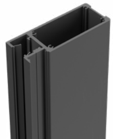
4 Heavy Duty Gate Frame 71" long Order Code: QSP-HDGATE-1828-FR • PP 534 / AP534 • .125" wall thickness with .2" center web • .125" radius corners
